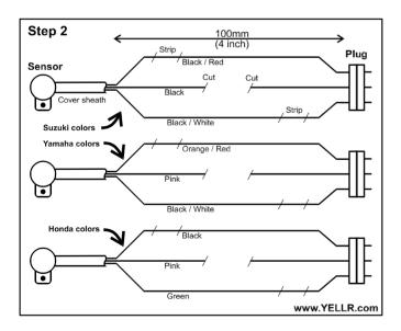
The wiring colors indicated above are for some Suzuki, Yamaha and Honda motorcycles. Your wiring colours may be different. Please check the **electrical diagram** in your vehicle's service manual and then confirm each wire with a **voltmeter**.
