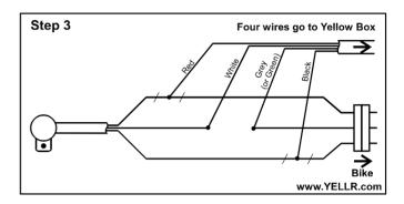
You must connect the Yellow Box wires exactly as shown above, or your speedo may not work properly. Carefully **compare your work** to the Step 2 and Step 3 pictures, and with the before and after diagrams on page 1.
