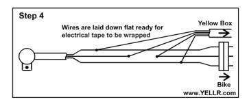
The diagram below shows the wires layed down flat - this is why we put 20mm (3/4 inch) between each connection, so now we can wrap electical insulating tape around this entire "bare" section to make it neat and safe again. Overlap the tape as you wrap it, check the other wiring in your vehicle and do it like that.
